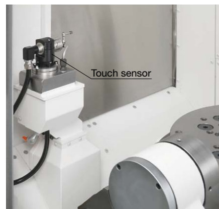
Tool breakage detection/Automatic tool compensation
